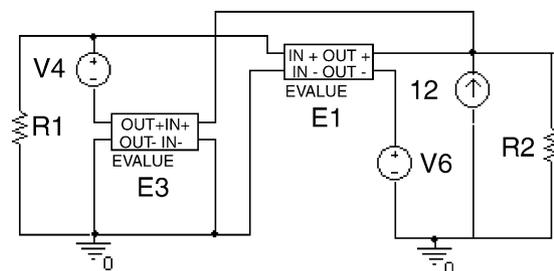
Fig. 2. Complete PSPICE ABM for NTCT with selfheating effect.  $VALUE(E1) = I(V6)R_N \exp[\beta/(V(IN1+, IN1-) + 273) - \beta/298]$ ,  $VALUE(E3) = I(V6)(V(IN3+, IN3-)/\delta)$ .
