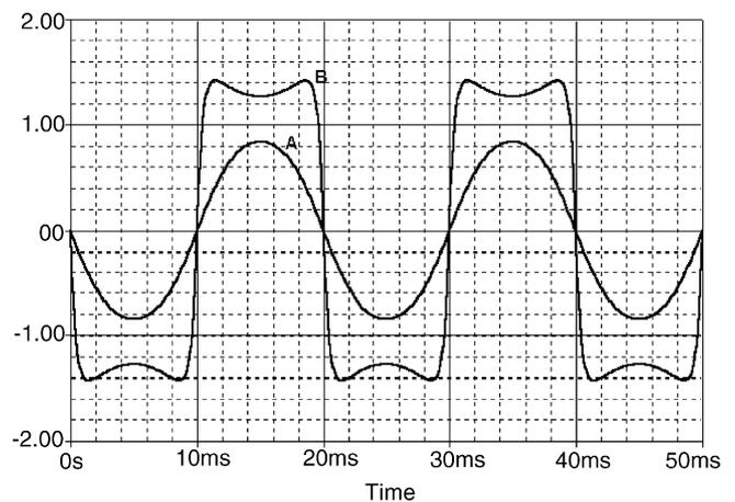
Fig. 5. Time domain transient analysis of the NTCT ABM for two sinusoidal currents of the same frequencies ( $50 \text{ Hz}$ ) with different amplitudes, in still air at  $25^\circ\text{C}$ . (A)  $I_{\text{max}} = 0.1 \text{ A}$ , (B)  $I_{\text{max}} = 1 \text{ A}$ .
