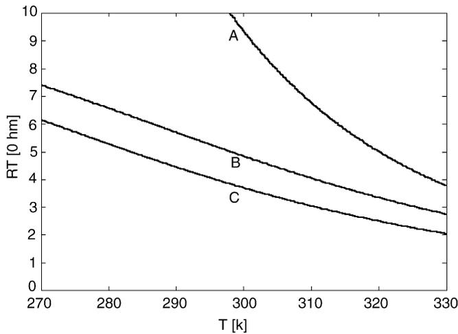
Fig. 3. Resistance vs. temperature curves of (A) unloaded NTC thermistor,  $R_N = 10 \Omega$ , without linearization, (B) same NTCT linearized by a parallel fixed resistor of  $10 \Omega$ , under no-load conditions, (C) same NTCT with a current  $I_T = 200 \text{ mA}$  and in parallel with a fixed resistor of  $10 \Omega$ .
