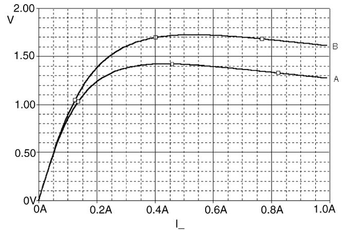
Fig. 4. PSPICE reconstructed current-voltage characteristic curve obtained from the NTCT ABM proposed in Fig. 2. The curve A is for  $\delta = 17 \text{ mW/K}$  in still air, while B is for  $\delta = 25 \text{ mW/K}$  non-conductive liquid. Ambient temperature is  $25^\circ\text{C}$ .
